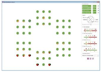
One of the most important steps of data analysis is determining which electrodes show stable signals. NOTOCORD-fps provides automatic electrode rejection by applying user defined criteria (beat rate, beat classification, etc.) to the first analysis period. Unsuitable electrodes are not included in the analysis, increasing accuracy.
