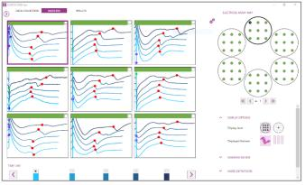
Once you import the data files, NOTOCORD-fps will return the analysis and results without any user interaction. A 6 well plate (with 54 electrodes, 5 sub-records, 10ks/s) can be imported and analyzed in less than 15 minutes!
