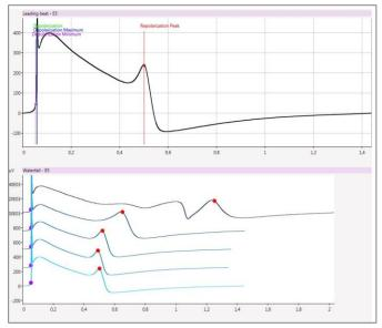
To improve marking quality, NOTOCORD-fps provides a user-friendly interface to quickly adjust a group of related marks by changing a single point on a single beat. The change will be applied to subsequent shapes automatically.
