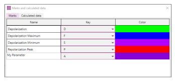
NOTOCORD-fps allows the user to define up to 26 characteristic points including all derived calculations (amplitude, duration, slope, etc.). Marks of interest are placed on reference beats from the first analysis period and propagated throughout the signal.
